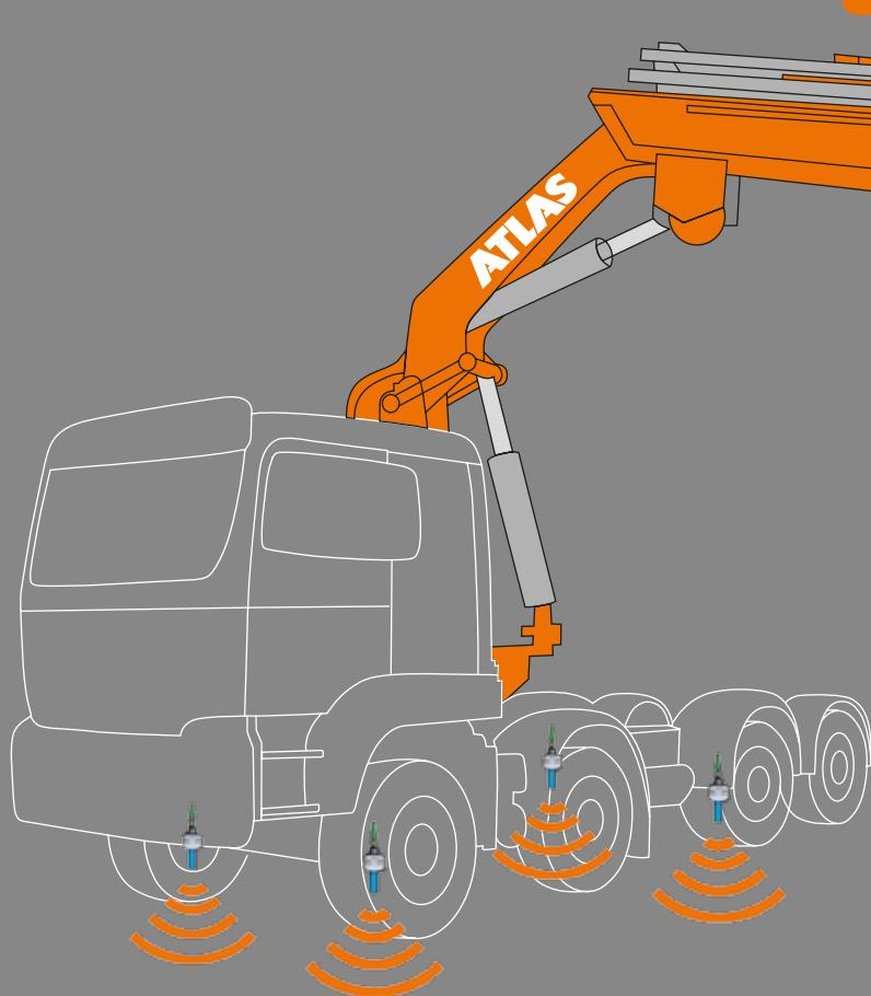
Four special ultrasonic sensors guarantee secure ground contact of the wheels and thereby the stability of the truck with loading crane
