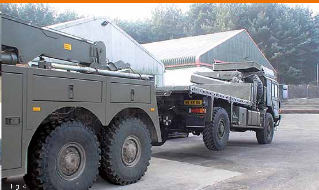
Fig 4 | Rear suspend tow. MAN 6 tonne Cargo during System integration trials.
