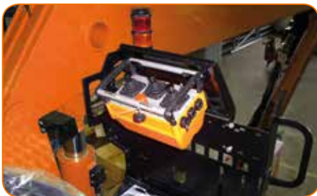
Seat on the column with a holder for radio remote control. Heatable shell seat upon request.
