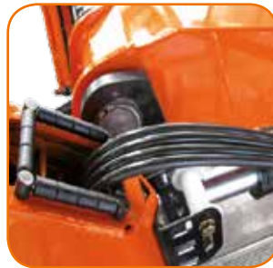
Internal hose routing, good protection for hoses.
