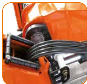
Internal hose routing, good protection for hoses.
